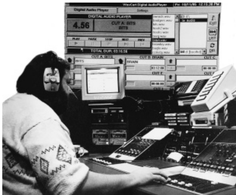
Figure 83 The virtual cart machine. Audio clips (actuality) are edited digitally and stored on computer for playback into news bulletins. The interface resembles an old-fashioned mechanical cart machine. ( Andrew Boyd )
