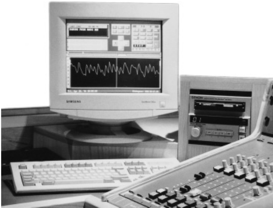
Figure 86 Revolution or evolution? Analogue faders, a cart machine and computer audio sit cheek by jowl. Sound is displayed on the monitor as a waveform. The 'tape' is shuttled back and forth by clicking on a button on the screen. Cutting and pasting is carried out electronically without a razor blade or chinagraph in sight. ( Andrew Boyd )
