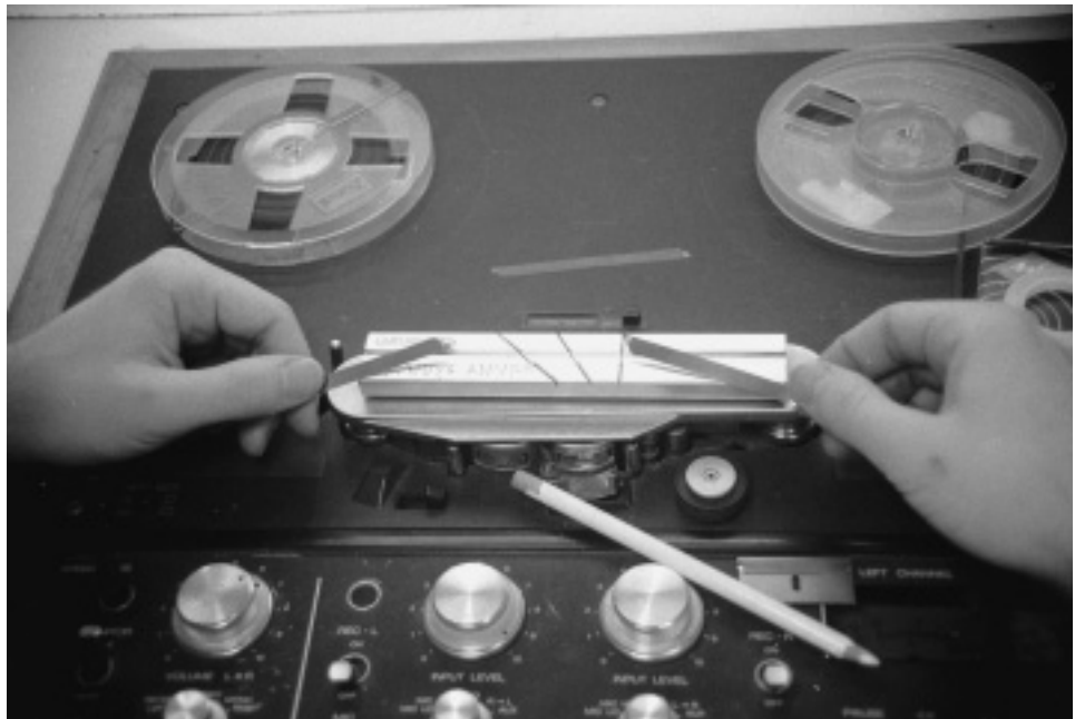
4 The two ends are butted together on the block to be joined. The unwanted portion – in this case a slight hesitation during an interview – can be seen above the editing block in the picture.
