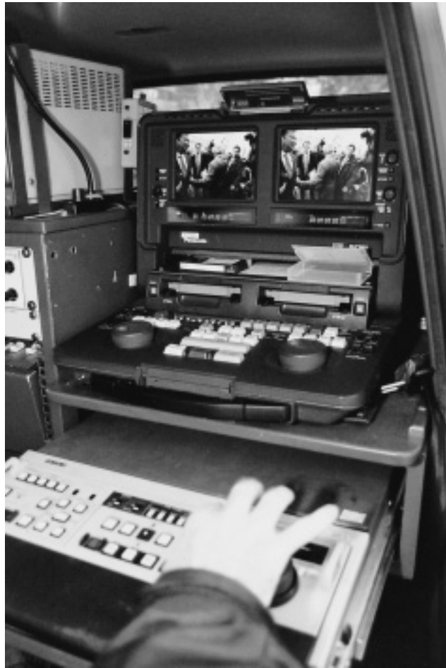
Figure 124 Panasonic linear digital editing system, as used by ITN. A kit the size of a small suitcase can be up and running in minutes, using miniature DV tapes. ( Andrew Boyd )
