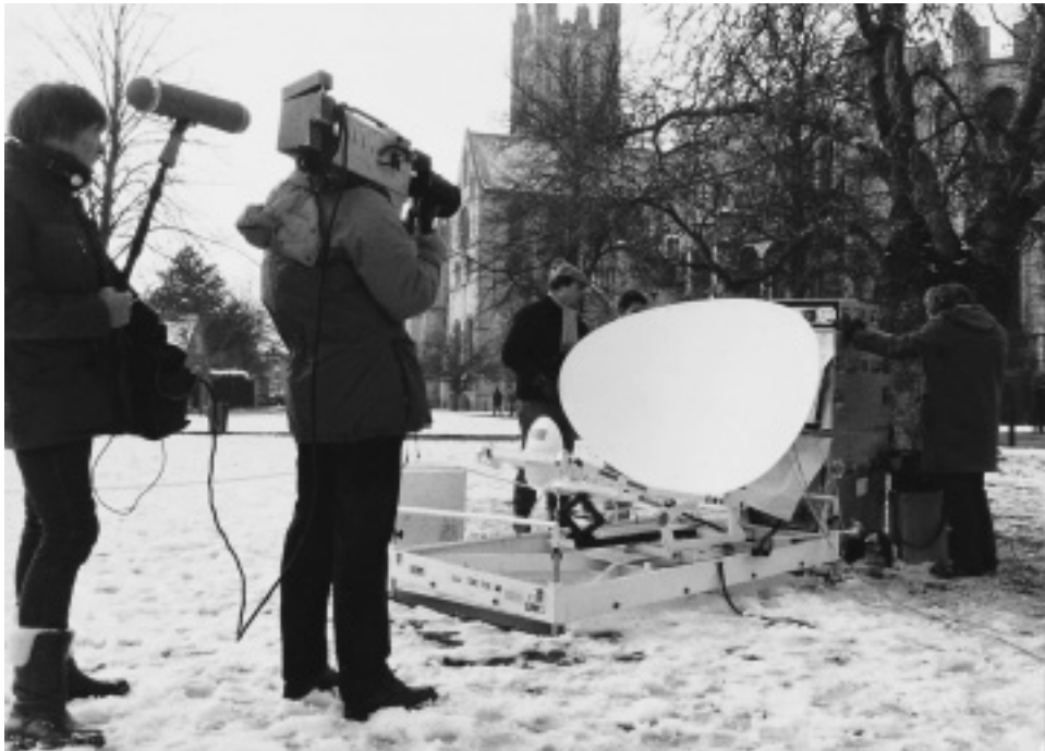
Figure 110 Portable ground-stations are used to beam news reports into space, where they are bounced off satellites and relayed to transmitters elsewhere in the world. ( Courtesy ITN )
