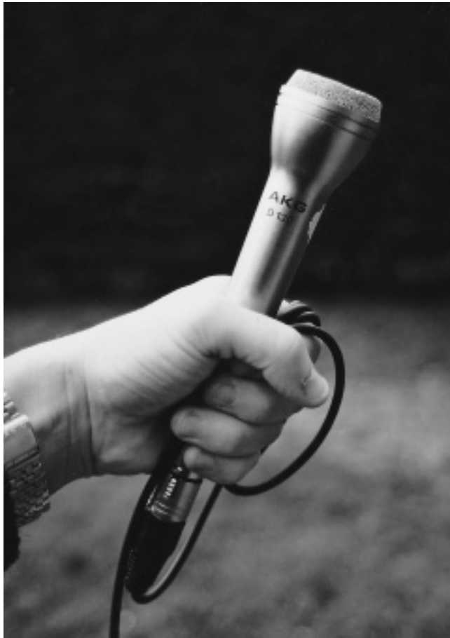
Figure 76 Where all it all begins – with the microphone. Take up the excess slack on the cable without tugging at the connection into the mike or into the recorder. Hold the mike firmly but lightly. Keeping your fingers still, tilt the mike towards whoever is speaking. ( Andrew Boyd )
