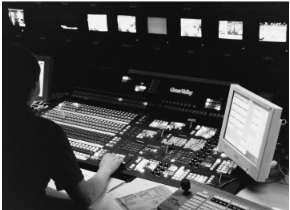
2 T-bars on the mixing desk dissolve from one input to another. The monitors are in black and white to give a crisper focus.
