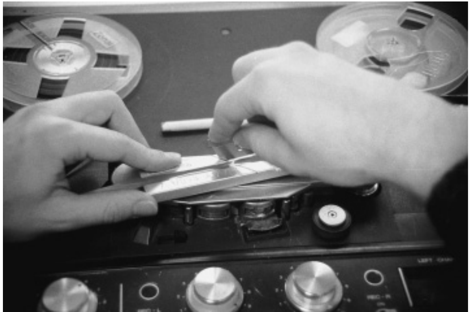
3 The unwanted section is cut out with an open razor blade (mind your fingers!) or a splicing machine.
