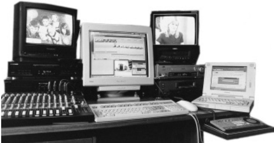
Figure 125 Desktop editing on a non-linear computer system. A setup like this costs a fraction of similar TV studio gear. Comprising (clockwise) sound-mixer, cassette deck, minidisc deck, monitor, NLE computer system running Adobe Premiere, second monitor/VHS deck, SVHS deck, DV input and edit deck, and laptop for writing the script. ( Andrew Boyd )
