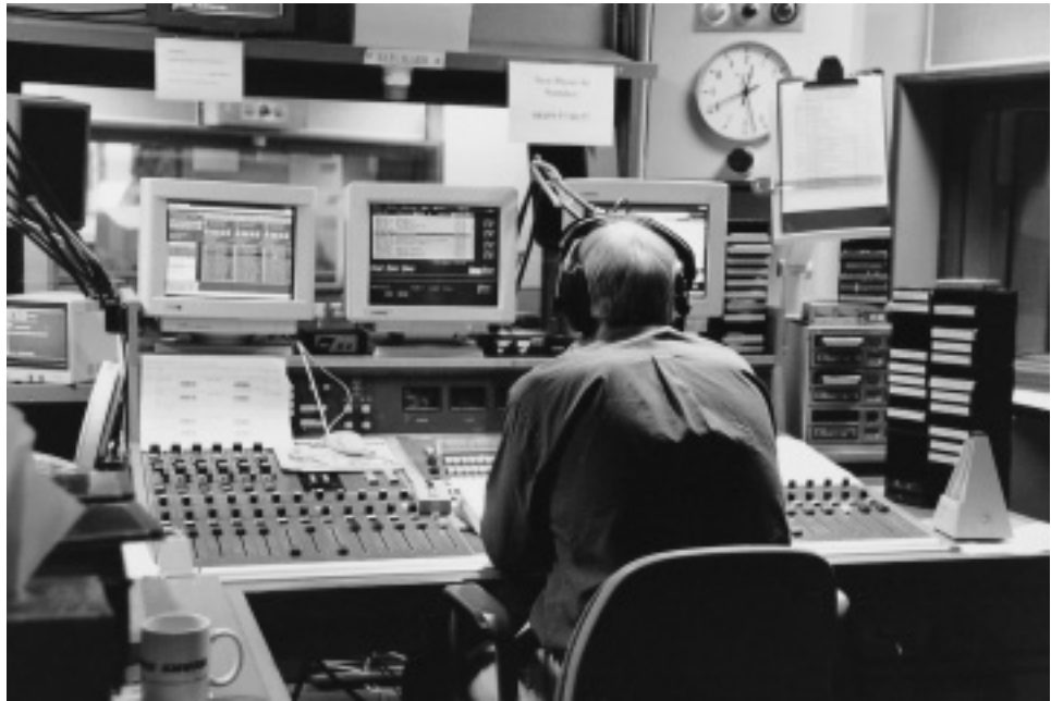
Figure 91 Catering for every form of audio, old and new – computers, phone, CD, cart, record and tape decks all input through the mixing desk at BBC Southern Counties Radio. ( Andrew Boyd )
