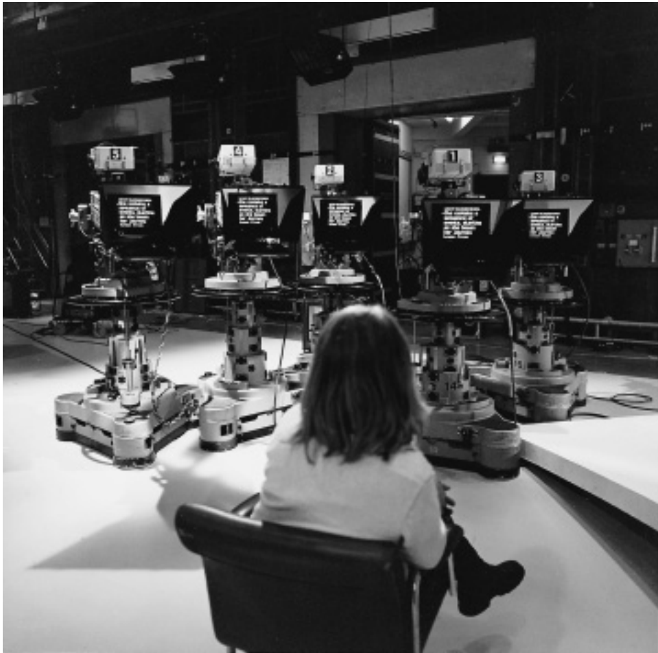
Figure 130 The anchor's best friend, the prompter. An operator controls the speed at which the script runs across the screen. (Courtesy EDS Portaprompt)
