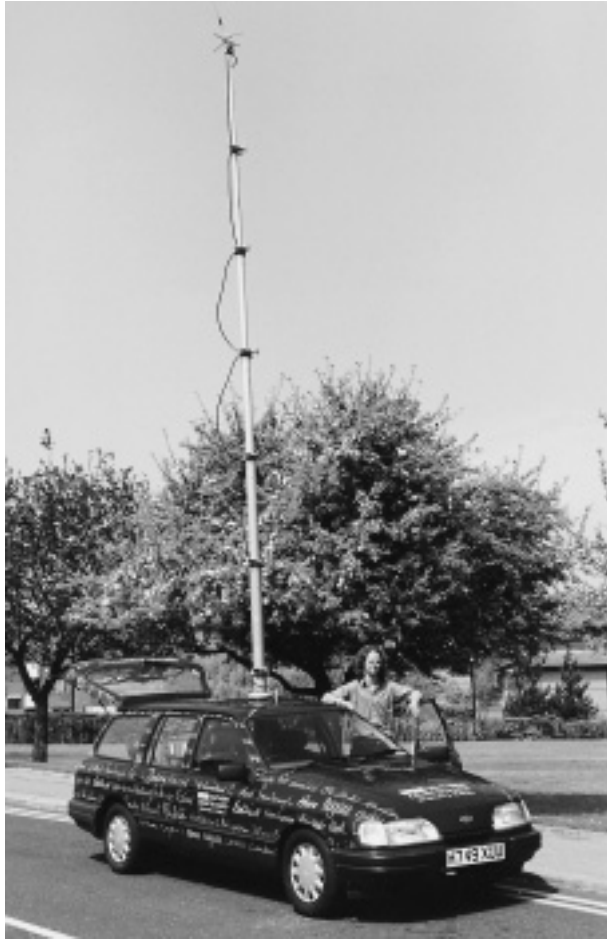
Figure 74 The radio car with its tall pump-up aerial acts like a mobile studio for sending on-the-spot reports back to the station. The idea is to keep the operation as simple as possible so that even the most non-technical of reporters can cover a breaking story without having to bring an engineer along to press the buttons. ( Andrew Boyd )
