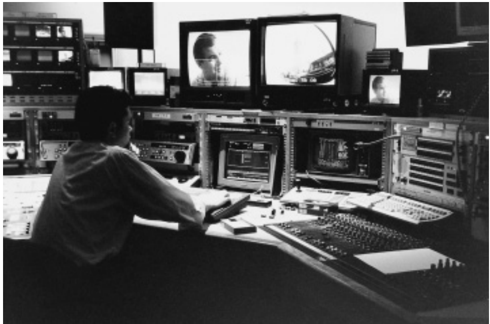
Figure 48 In the production suite. Computer-controlled editing lays down pictures, soundtrack and graphics directly onto the Betacam videocassette. (Andrew Boyd)
