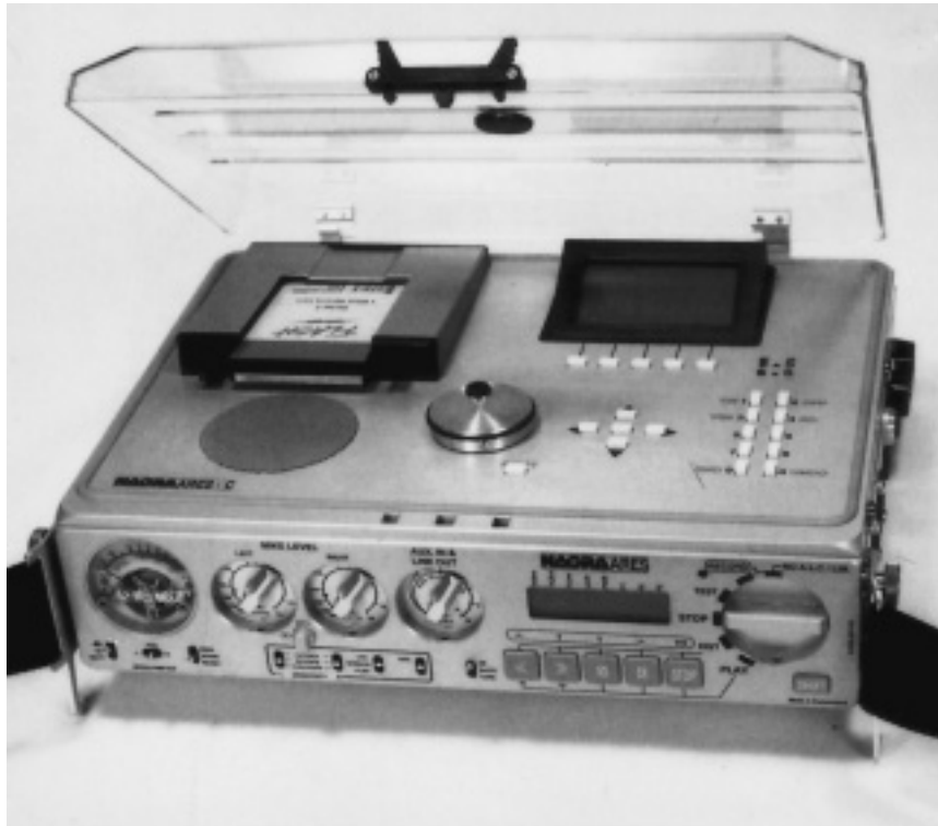
Figure 79 Getting more advanced – the solid-state recorder. This marvel from Nagra uses credit card-sized flash memory to store recordings. Interviews can be edited on the machine and downloaded directly onto a computer. No more moving parts. (Courtesy Kudelski)
