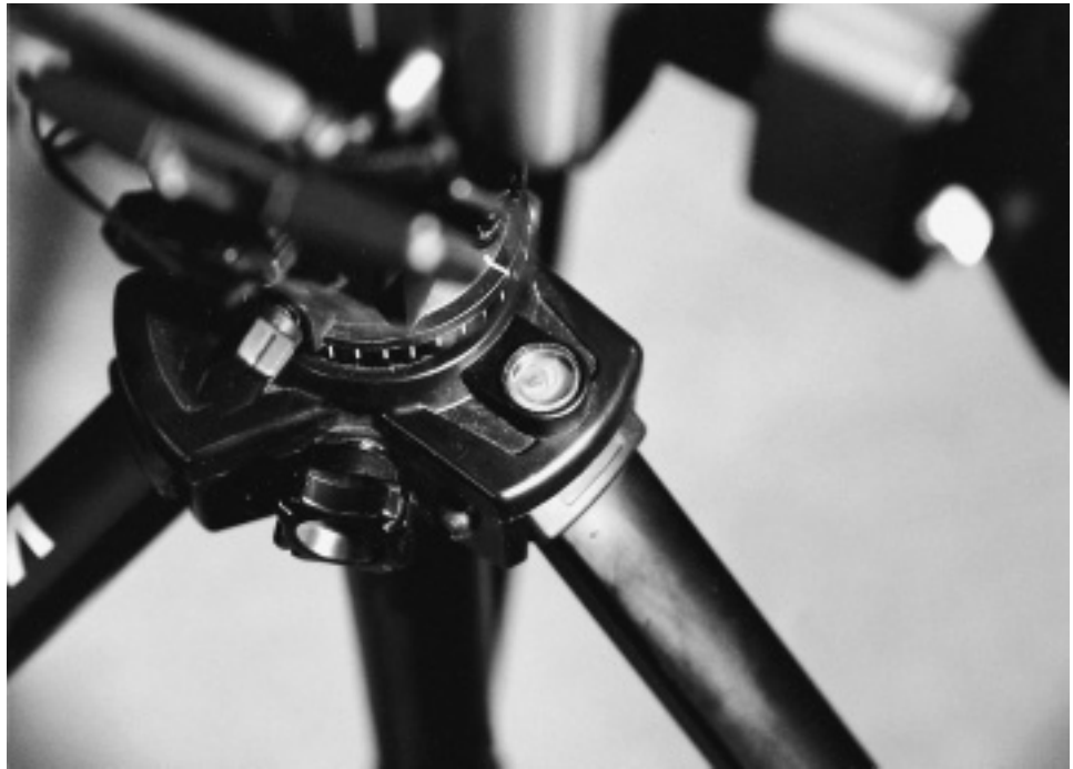
Figure 135 Tripods come in two flavours – those with legs you have to adjust individually, and those with self-levelling heads. The latter are faster to set up for the bustling VJ against a deadline. Use the button spirit level to make sure the camera is on an even keel. ( Andrew Boyd )
