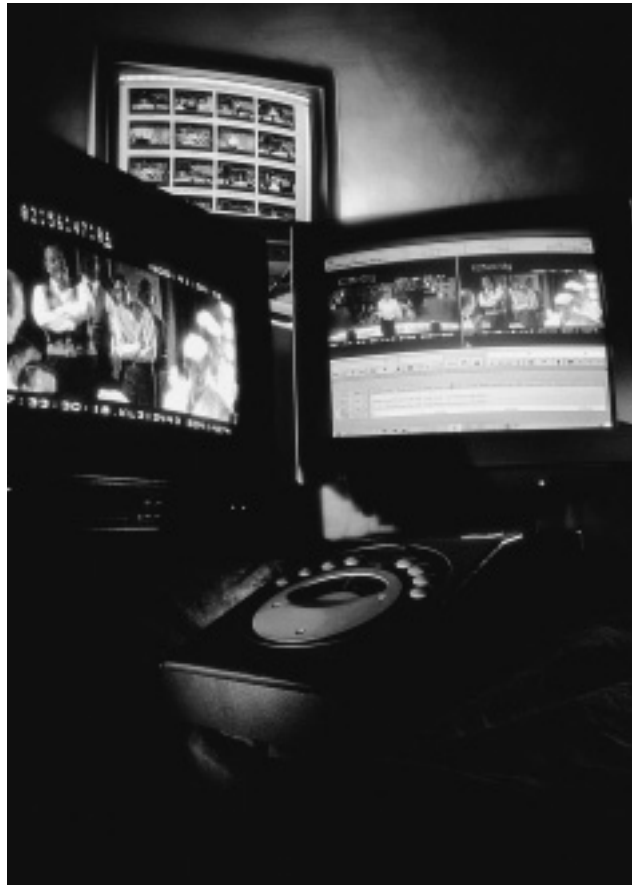
Figure 121 Digital images are edited on computer. The top screen shows thumbnail images of scenes that have been stored. They can be assembled in any order to produce an edited report. ( Courtesy Avid )
