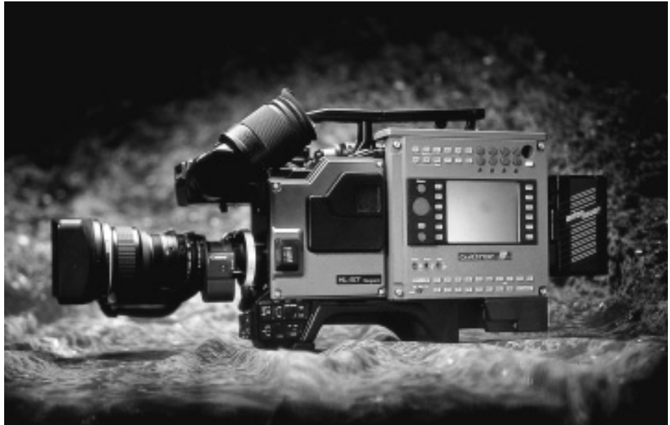
Figure 122 The Avid Camcutter rejoices under the title: tapeless field acquisition system . It's a digital camera that records directly onto hard disk. It means pictures can be accessed instantly. (Courtesy Avid)
