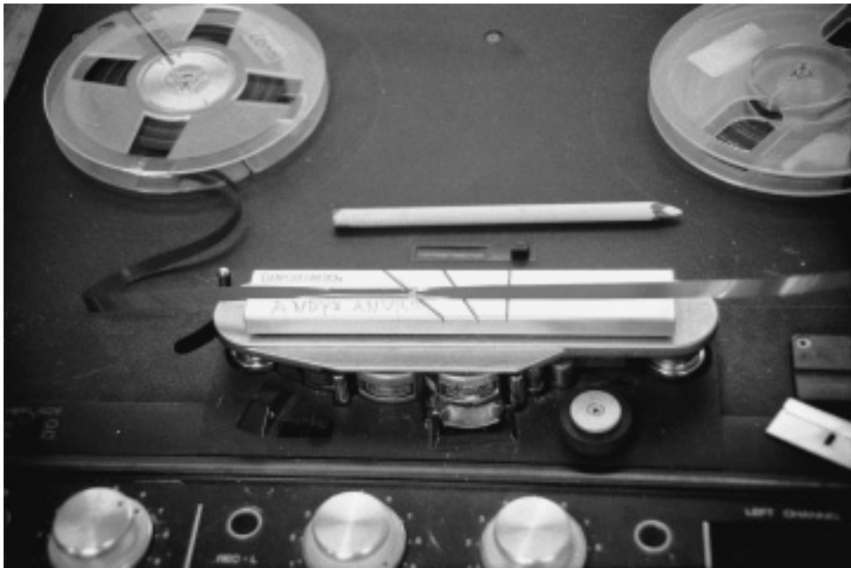
2 The mark is placed over the cutting slot on the editing block. The vertical cut is used for tight (close) edits.
