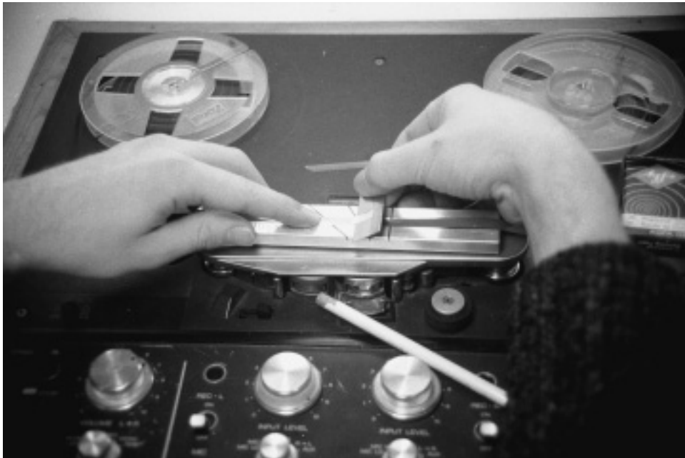
5 A short length of splicing tape joins the edited sections.
