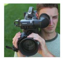
The shoulder-mounted handheld camera is steadied by the right hand, positioned through the strap on the zoom lens. That same right hand also operates the record button and the zoom rocker (servo zoom) switch.
