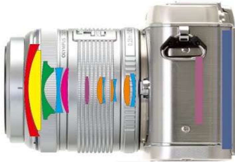
The internal structure of a MILC
