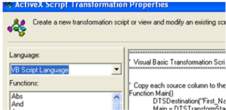
Slide shows the interface within the designer to write and test scripts that are written for transformation. Language dropdown menu on the extreme left corner allow us to select options available for scripting the transformation. As we are using VB scripts therefore make sure that VB Script should be selected in the dropdown menu.
