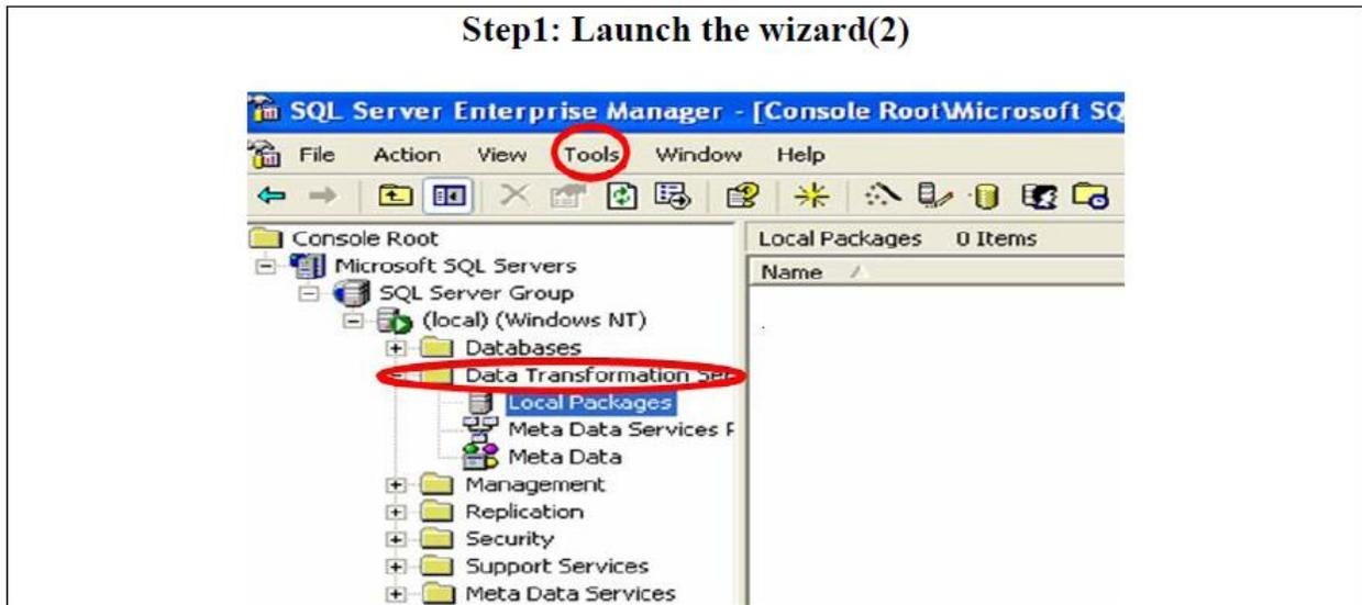
The slide shows the main screen of SQL Server enterprise manager. In the left pane we have Console root. We can see Data Transformation services highlighted. Expand the node mentioning Data Transformation Services and then press Tools in the menu bar. This will lead you to launch the wizard to load data.
