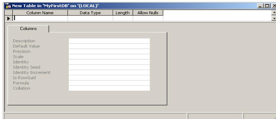
7. Type Column Name and select data type. See following figure in which we have created variable EmpID.
