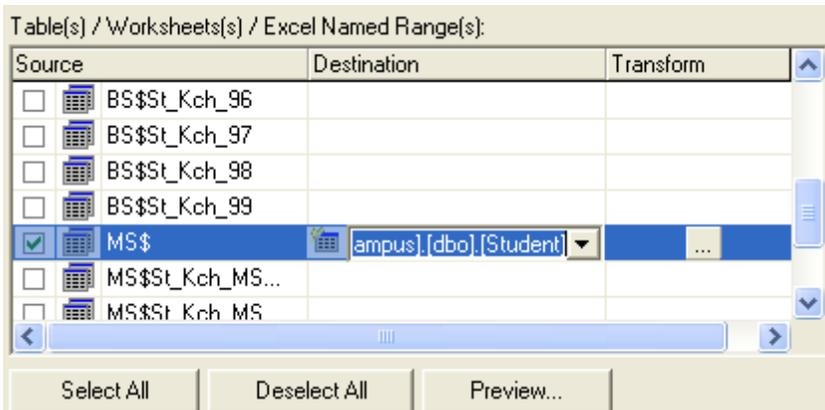
So, finally two options should be checked under the column Source, one is BS\$ and the other one is MS\$. Against both options the table name should be the same i.e. Student, because our destination is same. We can use third column transform, by pressing button against the selected row. This option provides us the same mapping view that we have seen earlier, while loading text file.
