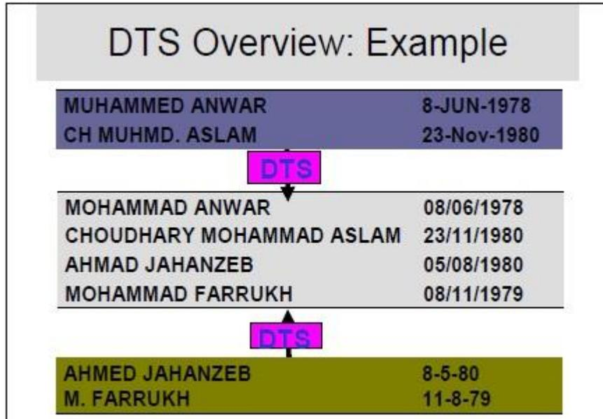
In this slide we may see three data management systems. Data is extracted from two systems, top and bottom, and is loaded into the standardized system shown in the middle. We may see two transformations over here.
