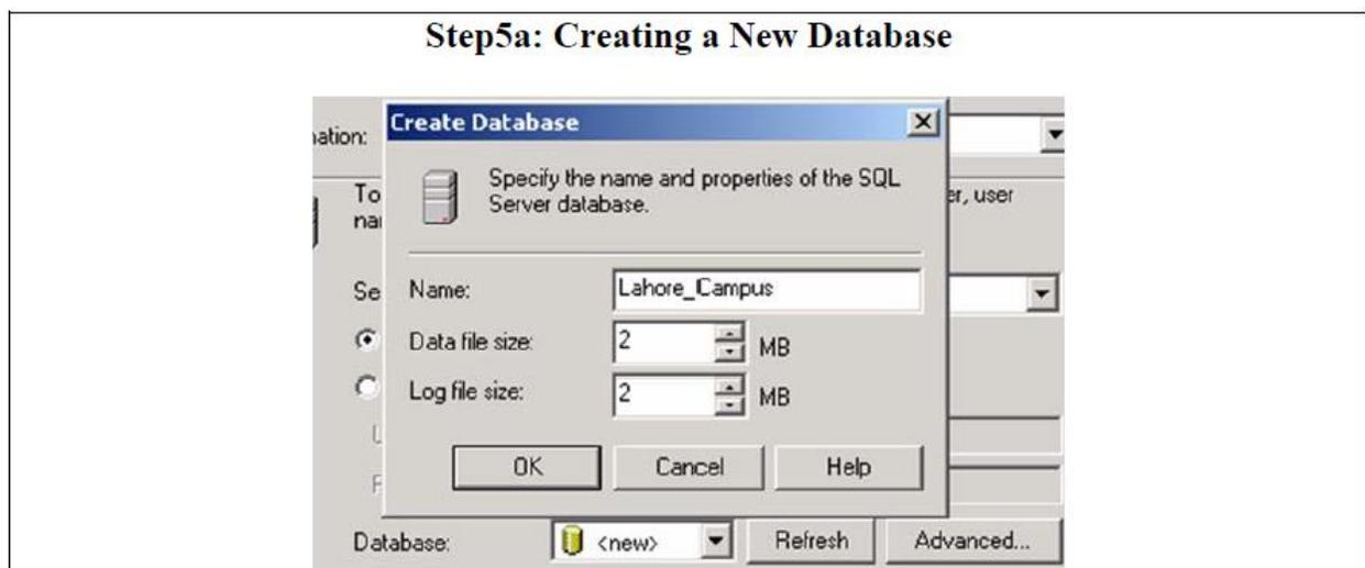
On selecting <new> option we can see this Create database pop up dialog box. This dialog box is asking for the name of database and the space needed for that database. Write name as 'Lahore\_Campus' and then press OK. Then press NEXT
