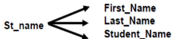
After SID we are required to transform St\_Name. It is one to many transformation that is required to be specified through script. In this case is source column is just one 'St\_Name' and the destination columns are three 'First\_Name', 'Last\_Name', & 'Student\_Name'. We are required to create three new transformations,
