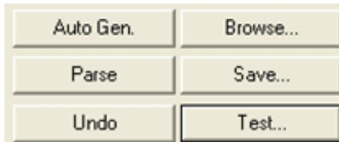
On the extreme left corner of the scripting interface dialog we can see six options as shown in the slide. We can save our scripts, we can browse them later on, we can parse them for syntax errors, we can undo last move, we can auto generate simple copy column script and we can test our scripts on actual column of database table. To verify the correctness of the script we can use **Test** option. Test option runs the script on the actual column and shows the first hundred values as an output.
