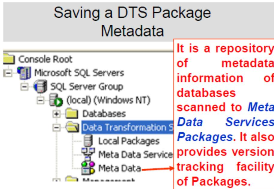
If a package is saved to SQL Server 2000 Metadata Services and is scanned for metadata than its meta data information is maintained in a repository "Meta Data ", that can be found as third option under node Data Transformation Services.
