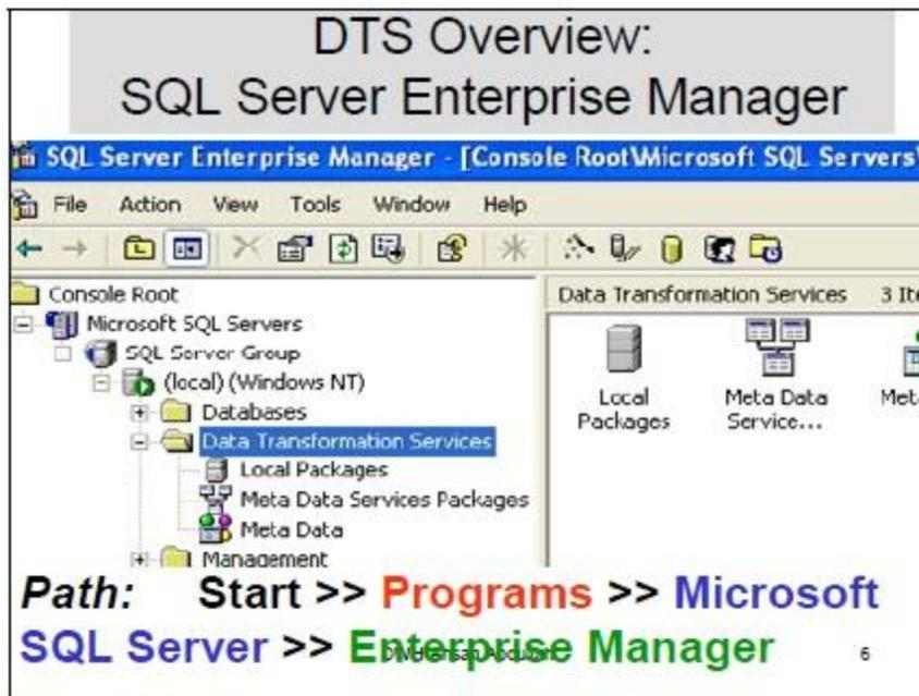
The Data Transformation Services (DTS) node of the SQL Server Enterprise Manager Console tree provides facilities for accessing DTS tools, manipulating DTS packages, and accessing package information. You can use these facilities to:
