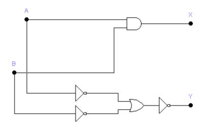
According to the circuit above find the equation of X and Y, then fill the truth table.
