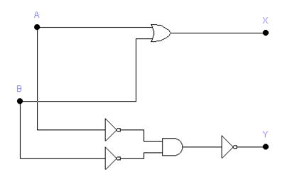
According to the circuit above find the equation for X and Y, then fill the truth table.
