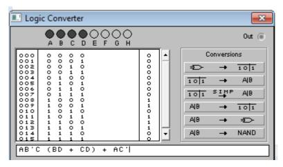
**Task 6: Simplifying Boolean functions in EWB using the logic converter** Simplify the following Boolean expression in EWB using the logic converter
