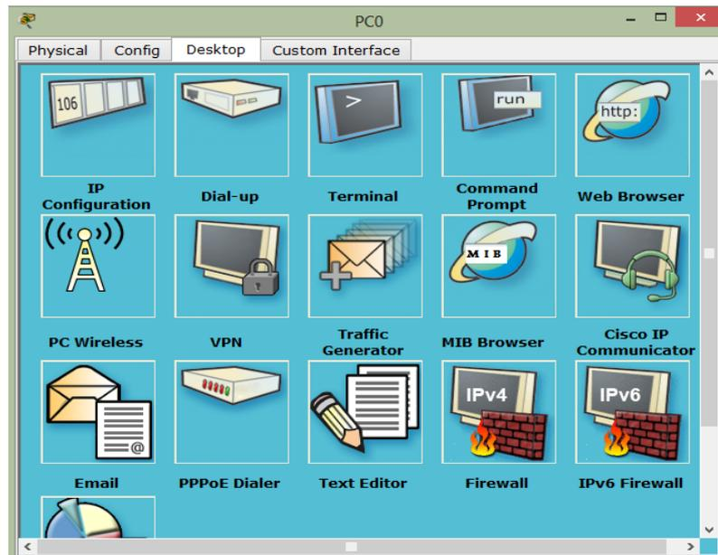
**IP Configuration:** With this utility, you can assign a dynamic or static IP address to an end device. If you choose to enter a static IP address, **Subnet Mask** field gets filled according to the class of the IP address. In case you want your devices to obtain IP dynamically, then choose **DHCP** here. Configure **DHCP** on **Server-PT**.
