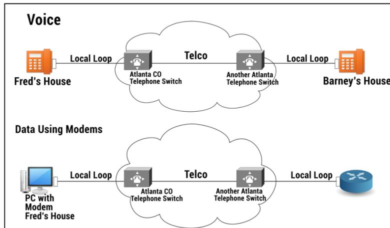
**Figure 72.2: Comparing a Phone to a Modem**
