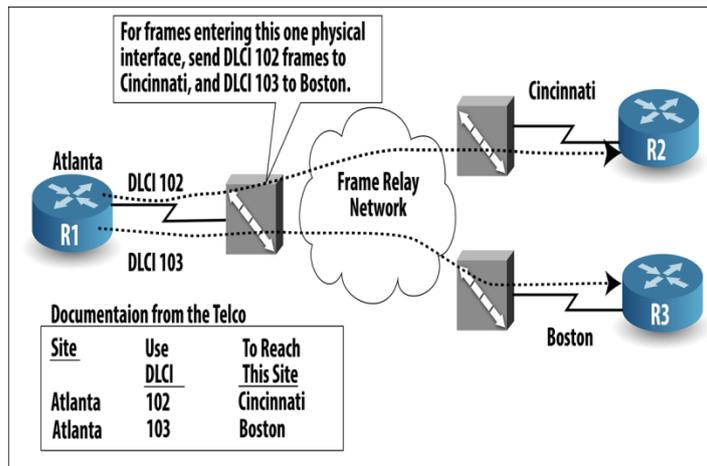
**Figure 68.1: Frame Relay Switching to Multiple Remote Sites**
