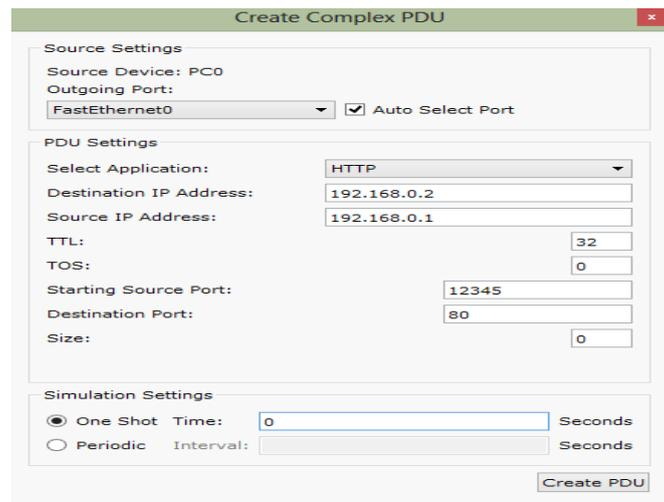
Select **application** as HTTP, fill the **Destination IP address** = 192.168.0.2, **Starting Source Port**, (let's say 12345), and **Time** = 0, and then click on the **Create PDU** button.
