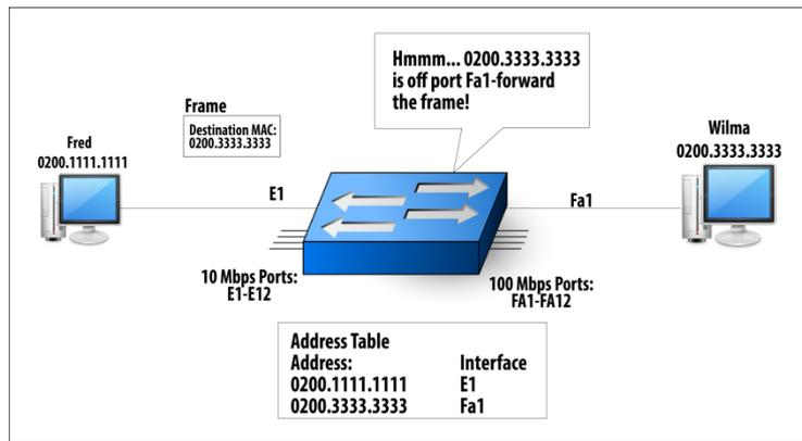
**Figure 24.1: Supporting Multiple Speeds on a Single Switch**
