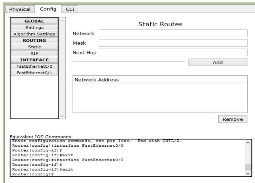
Dynamic routing such as Routing Information Protocol (RIP) can be configured by adding only the network IP.
