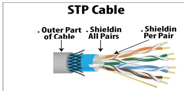
**Figure 13.2: Shielded Twisted Pair (STP) cabling**
