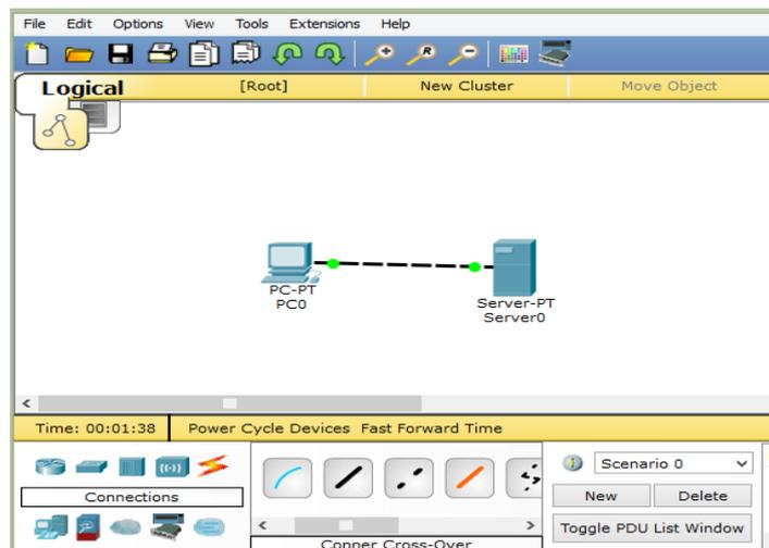
**Step 5:** Click on the **real time/simulation** tab and switch to the simulation mode.
