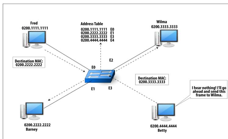
**Figure 22.1: Potential Collision When Forwarding Multiple Frames**
