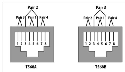
**Figure 13.4: Pinout options for (RJ 45) Connectors**
