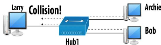
**Figure 15.2: Collision between Bob's and Archie's Frames**
