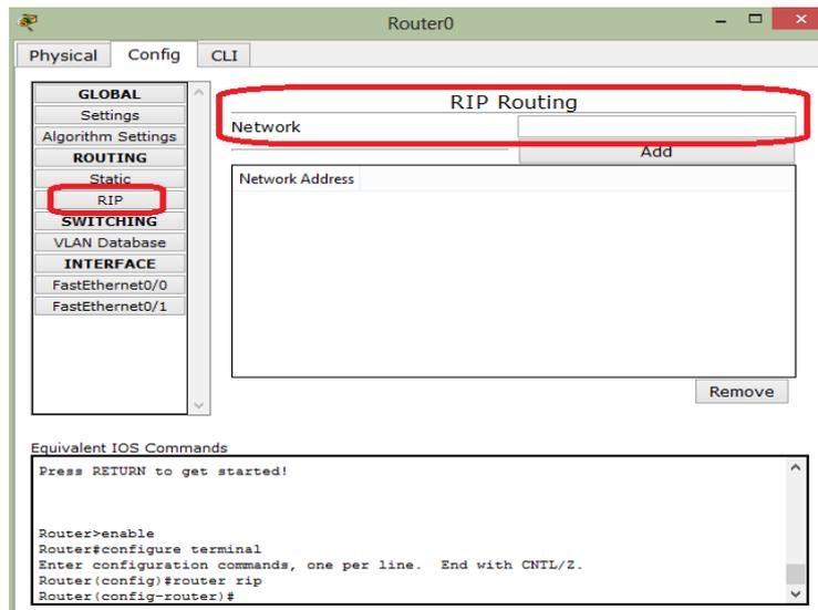
**VLAN database:** Available on a switch. It allows you to create and remove VLANs.
