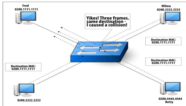
**Figure 21.1: Potential collision when forwarding multiple frames**
