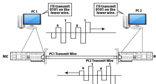
Figure 12.4: Concurrent Data Transmission across Two Different Wires
