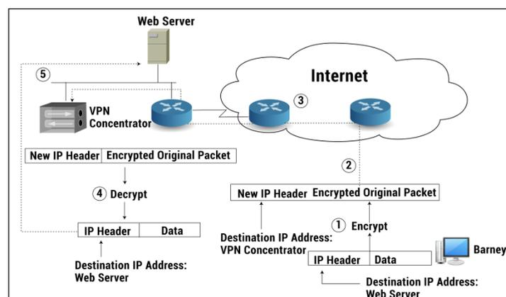
Figure 77.1: Encrypting IP Packets for a VPN
