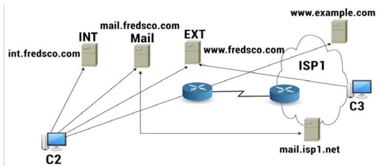
Figure 78.2: Typical Types of Traffic Between an Enterprise and the Internet
