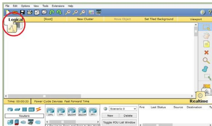
**Common tools bar:** With help of this toolbar, we can manipulate topologies. For example, select, move layout, place note, delete, resize shape, add simple/complex Protocol data unit (PDU).
