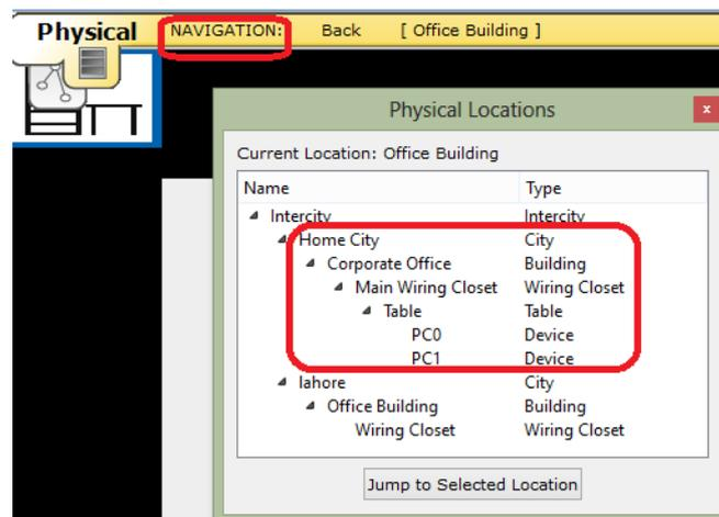
**Step 6:** Use the **Move Object** button and move one of the PCs to **Lahore | Office Building | Wiring Closet**.
