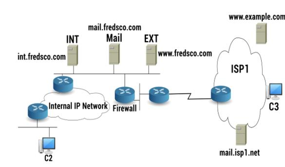
**Figure 79.1: Putting Up a Wall Between the Dangerous Folks and Your Network**
