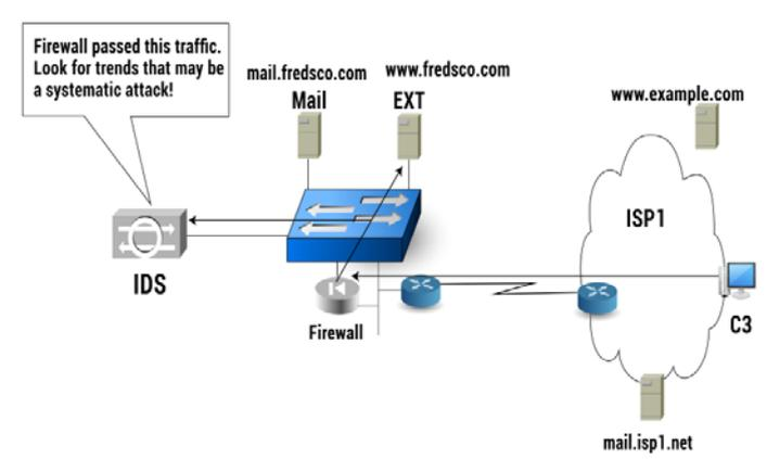
**Figure 79.6: Watching for Patterns with a Network-Based IDS**
