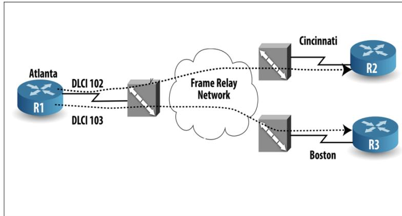
**Figure 69.2: Typical Frame Relay Network with Three Sites**
