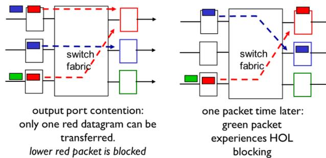
**Figure 53.6: The Head-of-the-Line (HOL) blocking at Input Port**
