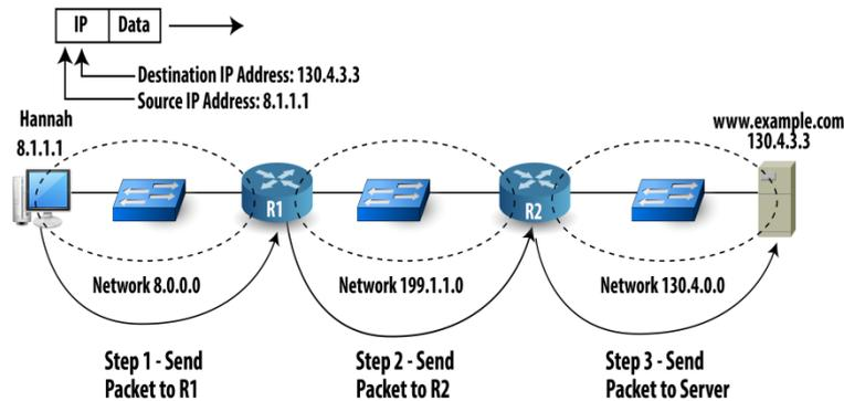
Figure 49.1: Working of Default Gateway Router
