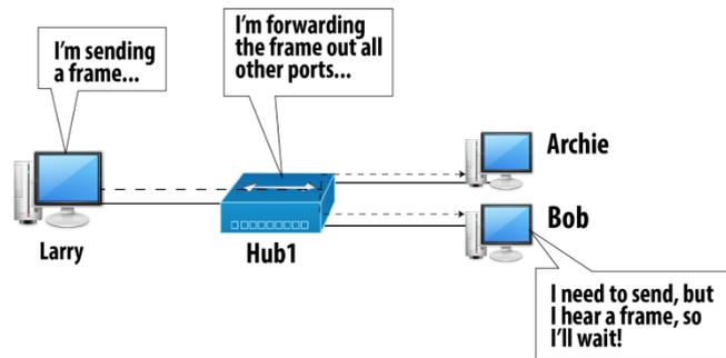
**Figure 16.1: Collision Avoidance by Listening before sending**
