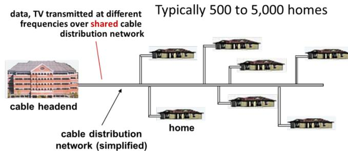
Figure 74.1: A hybrid fiber-coaxial access network
