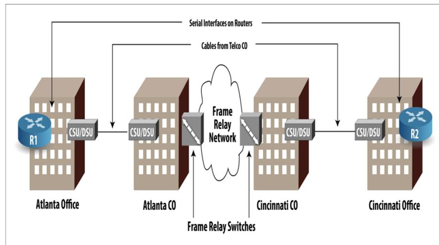
**Figure 66.1: Physical Parts of Frame Relay**
