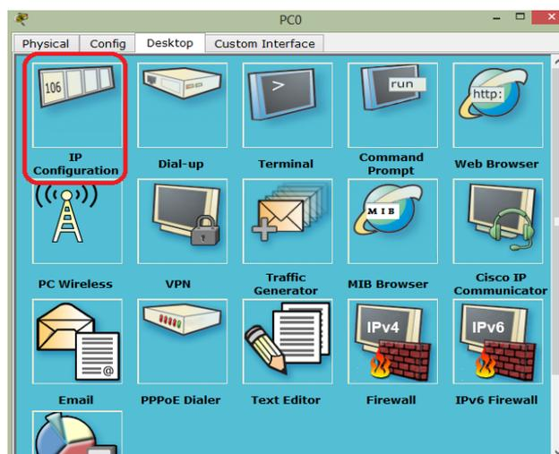
Click on **IP Configuration**, and enter an IP address and subnet mask. No information required for a default gateway and DNS server. Close the window
