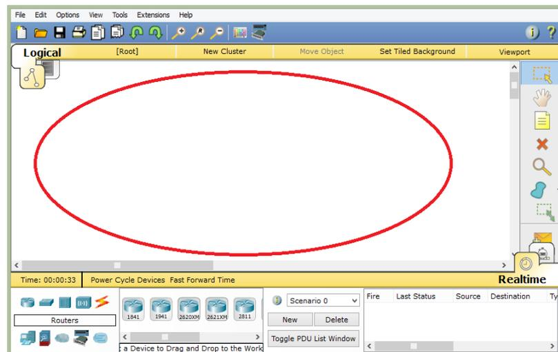
**Real-time/Simulation tabs:** With these tabs, the operating mode can be switched between the real and simulation modes. Buttons are also provided to control the time.
