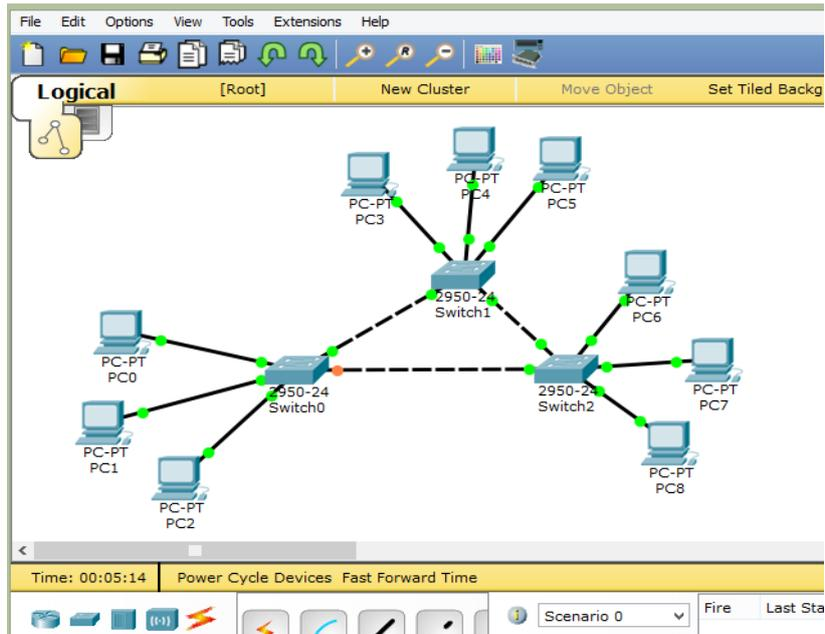
**Step 2:** Combine PC0, PC1, PC2 and Switch0. Select PC0, PC1, PC2, and Switch0 by clicking on whitespace. Click on the **New Cluster** button on the top-right corner.
