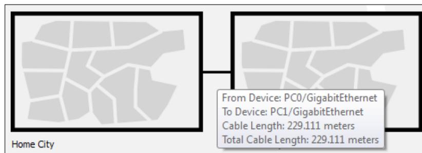
The length of Standard copper Ethernet cables can extend up to 100 meters. Let's test that the connection comes down due to the distance.
