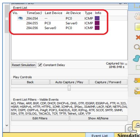
To view a packet's TCP/IP layers information, click on a packet (the envelope icon). The **Outbound PDU Details** tab lists each layer's information.
