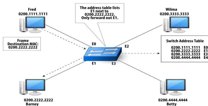
**Figure 20.2: Switch logic**
