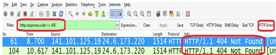
**Step 4:** Right-click on **Packet 61** and select **Follow TCP Stream**. This will allow us to figure out what item was not found on the server. **Follow TCP Stream** applies a filter based on the Stream Index number. Also, a window is opened that depicts the conversation without headers.
