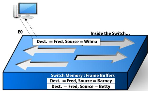
**Figure 21.3: Switch Avoids Collisions by Buffering the Frames**
