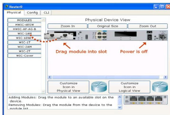
A module can be removed by first, powering off the device and then, dragging it from the slot back to the module list.
