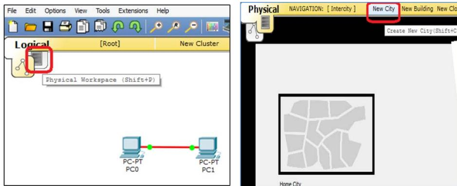
**Step 5:** Use the **NAVIGATION** button and go to **Home City | Corporate Office | Main Wiring Closet**. Both the PCs we inserted in the logical workspace are located here. Jump to their location.
