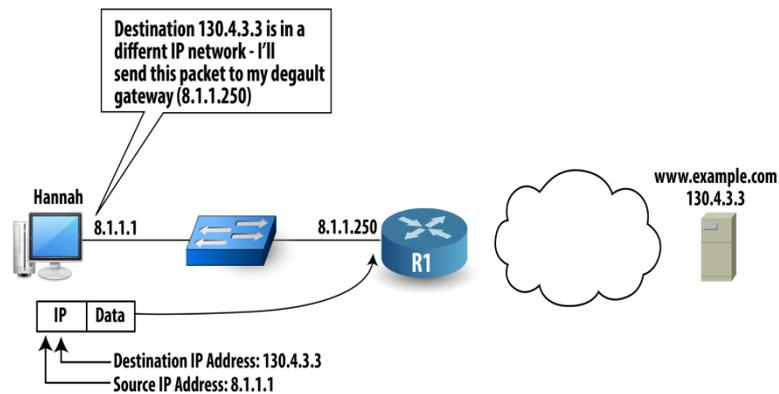
**Figure 49.2: Software of Hannah's PC has built the IP**
