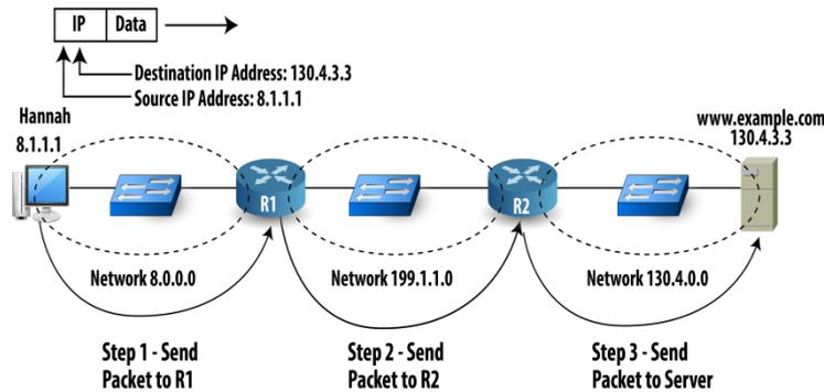
**Figure 51.1: Router's Routing Logic and Table**
