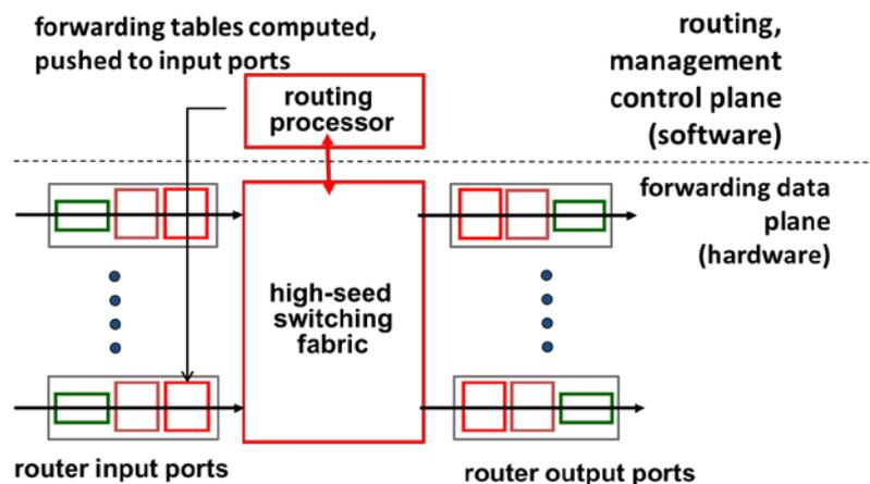
Figure 53.1: Router Hardware Architecture
