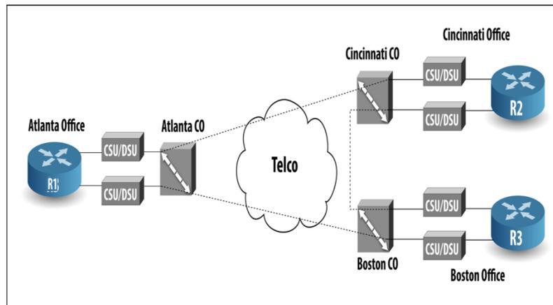
**Figure 69.1: Three Leased Lines to Connect Three Routers**
