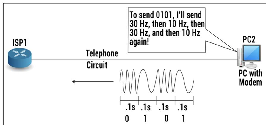
**Figure 72.3: Basic Operation of Modems over PSTN**
