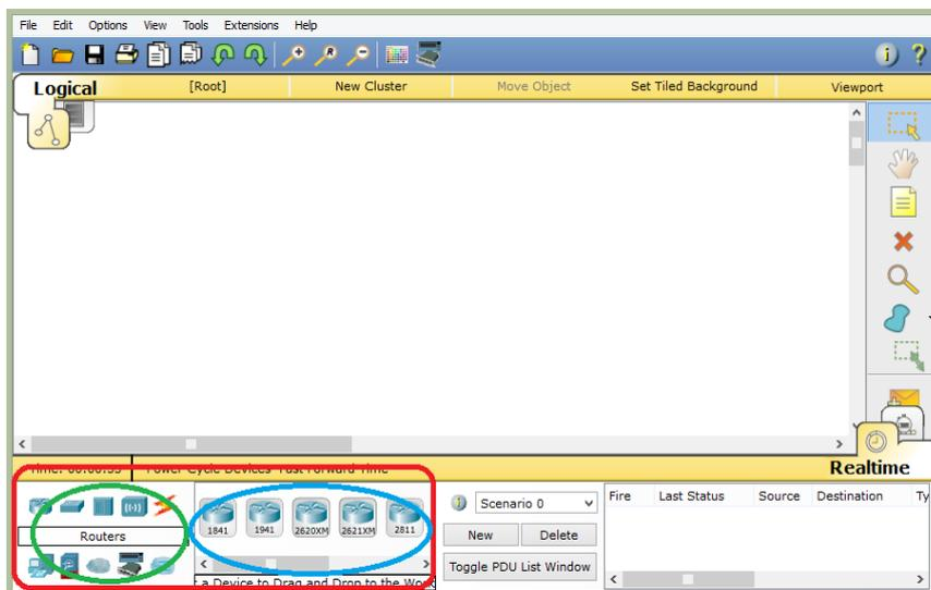
**Device-type selection box:** Device categories are given here.
