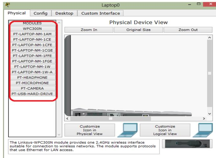
**Linksys-WMP300N:** Through this wireless interface, you can configure a WLAN.
