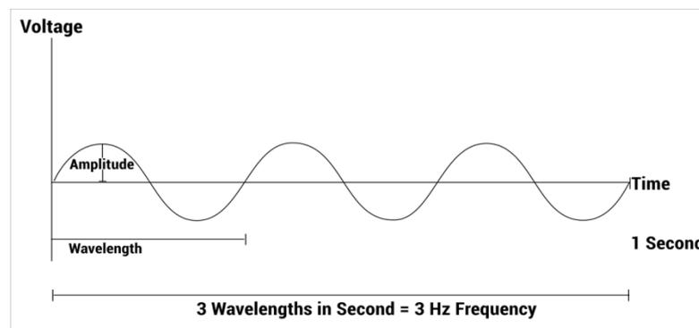
**Figure 72.1: Analog Electrical Signal: Frequency and Amplitude**
