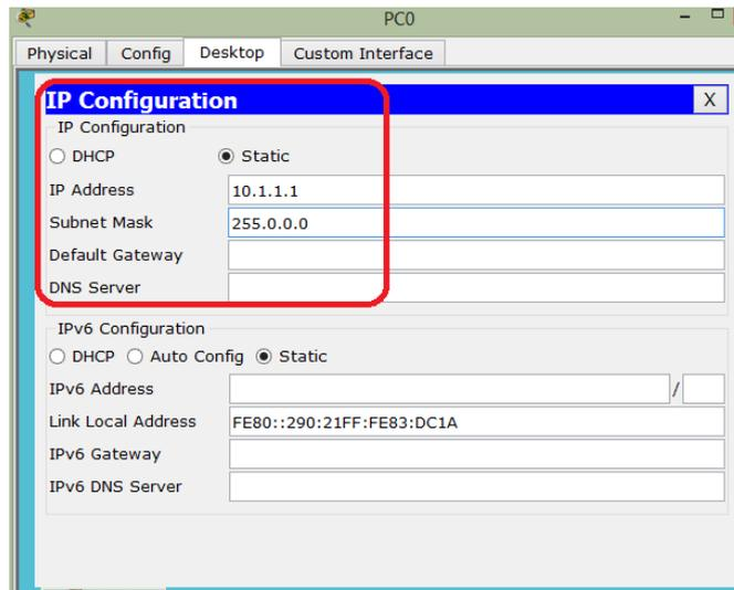
**Step 5:** Repeat step 4 for the laptop. Make sure that both of the IP addresses are in the same subnet.
