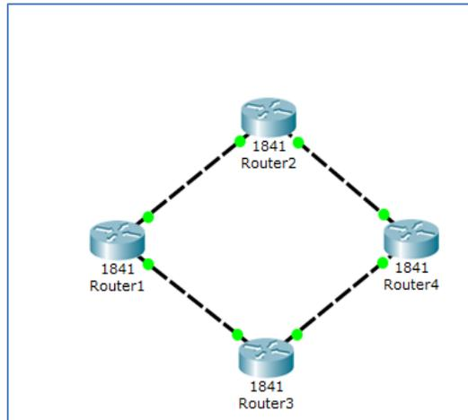
**Step 4:** Once the topology is configured, use the simple PDU to check for connectivity.
