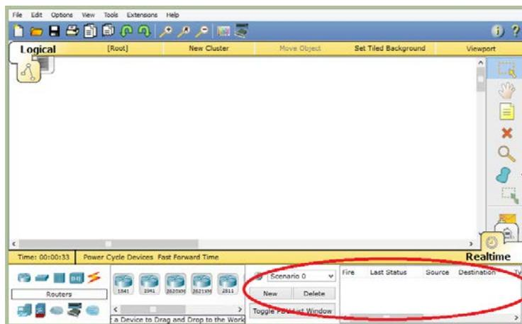
**Network component box:** All of the network and end devices available in Packet Tracer are listed in this component. It can be sub-divided into two areas:
