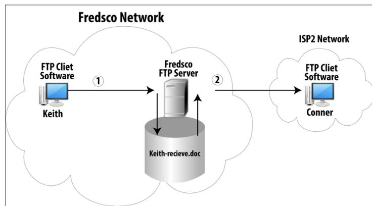
**Figure 30.2: FTP Process for Transferring Files**
