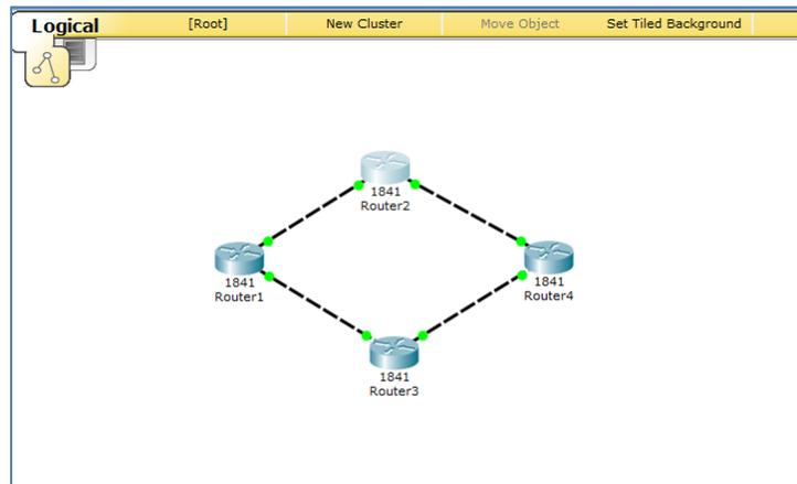
**Step 5:** Test the connectivity between all of the routers with the help of **simple PDU**. Click on a router first and then click on another router. Look at the **User Created Packet** box.
