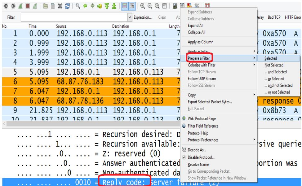
Using this filter will locate Server Failures. As we want to create a button to display DNS errors. All such packets will have values larger than 0 in the **dns.flags.rcode** field.
