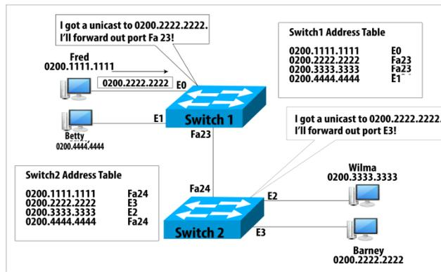
**Figure 27.1: Forwarding Frames Between Two Switches**
