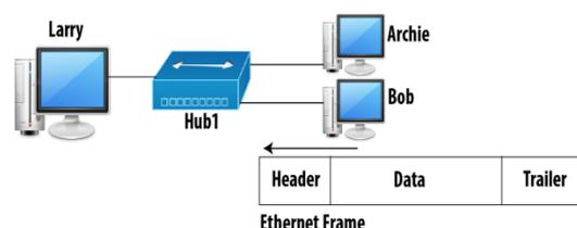
Figure 15.1: Ethernet Frame sent from Bobs to Larry
