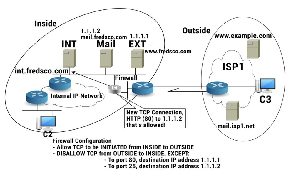
**Figure 79.4: Disallowing a TCP Connection to an Inside Web Server**
