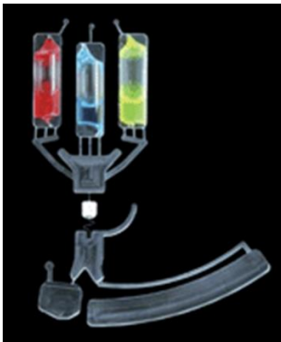
Fig shows Glass ampoules for reagent storage in Lab on chip.
