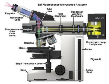
fluorochrome tagged antibodies. See the accompanying diagrams for details. Look for UV lamp (Mercury Lamp).
