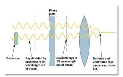
retarded light ray, a phase plate is inserted into the body of the microscope (above the objective lens) which is thicker in the center than the ends. This arrangement causes the
