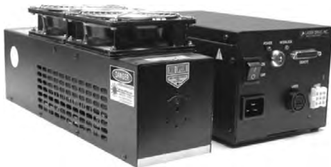
FIGURE 16.10 ► Argon-ion laser. From www.nationallaser.com
