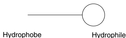
FIGURE 7.10 ► Schematic of a surfactant molecule.
