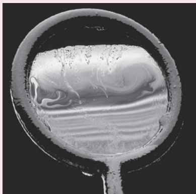
FIGURE 32.14 Interference in a soap film illuminated with white light.
