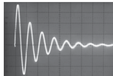
FIGURE 28.13 An oscilloscope displays the capacitor voltage in an RLC circuit.
