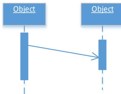
There are different types of messages between objects for interaction in the sequence diagram. These are synchronous, asynchronous, self message and return messages.
