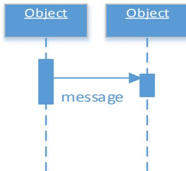
Message sending is usually assumed to be virtually instantaneous. However, in a situation where the message is sent over a communication link and a significant amount of time elapses between the sending and receiving of the message, the arrow can be shown slanting down the page like in the figure.
