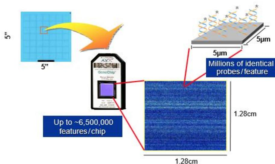
These GeneChip microarrays are a fusion of the technology of the semiconductor industry with life sciences – this is why these arrays are called “chips”. The chips are manufactured on wafers. These wafers are 5-inch-by-5-inch pieces of glass. You can get anywhere from 49 to 900 individual chips out of each wafer, depending on the overall size of the final chip to be made
