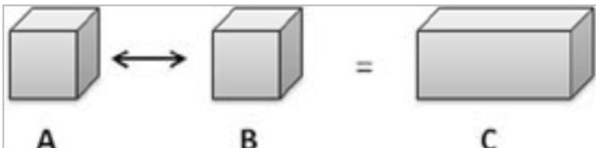
The surface energy of two separate cubes is higher than the surface energy of the two cubes agglomerated. Nanoparticles have a strong intrinsic tendency to agglomerate. To avoid this, surfactants can be used. This also explains why when nanoparticles are used in research and industry they are often immobilised on a solid support
